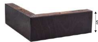
W02, Plywood, painted black
